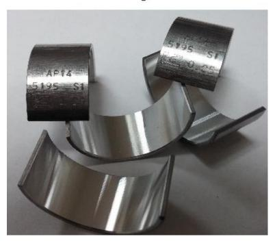
A bimetal structure with an aluminum alloy lining is the best solution for camshaft bearings. Aluminum alloy is not too hard, therefore it has good conformability. On the other hand it is stronger and more wear resistant than babbitt.
